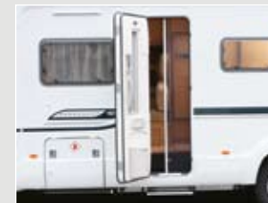
Entrance door Entrance door with secure 3-point locking, hidden hinges, double seal system and stepwell light
