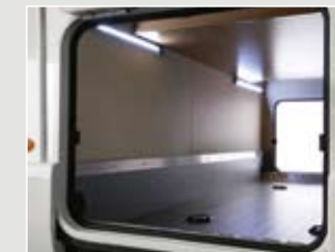
Lighting in underfloor storage trays Underfloor storage trays provided by the Fiat/AL-KO low-line chassis with 190mm (7½") double floor have lighting
