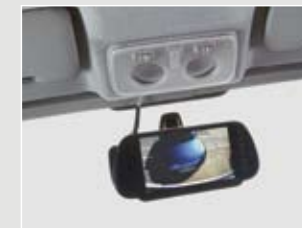
Reversing Camera Reversing camera with image shown on rear view mirror
